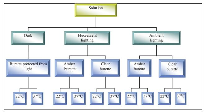
Figure 1 Schematic representation of the experimental design used in the analysis of pH with various exposure times, luminosities, and temperature conditions.
